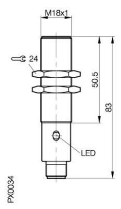
**Inductive Sensors** BES 516-326-G-S 4-H M18x1 x 83 normally-open Sn=8mm shielded
